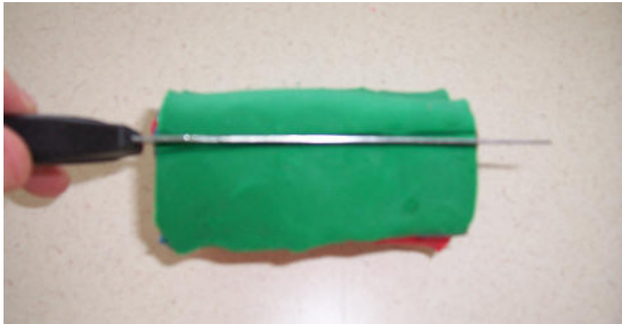
Step 6: Non-plunging folds. Cut clean across the top creating nice parallel bands.
